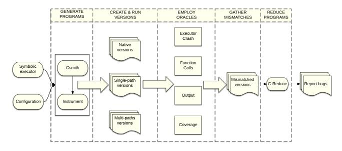
Fig. 1. The main stages of our testing approach.
